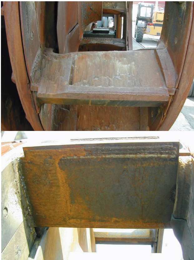
Figure 5. Impact plate with typical wear pattern (top) and partial new hardfacing (bottom).
