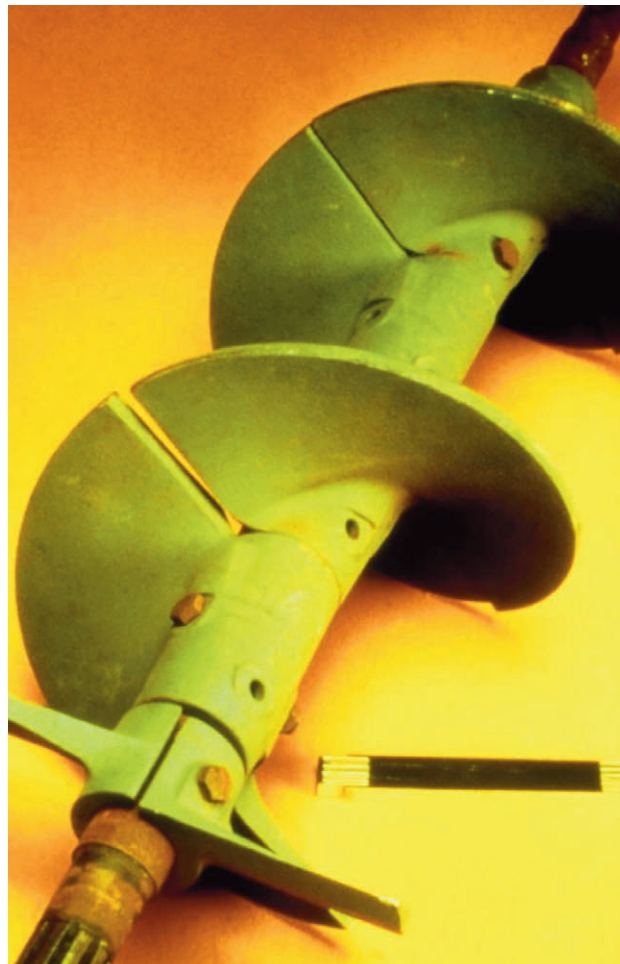
Figure 3. Screw conveyor with cast iron spiral.
