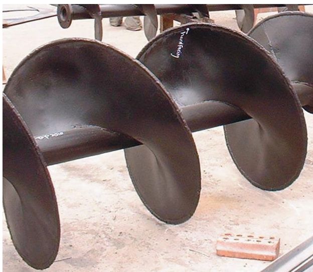
Figure 2. Screw conveyor with spiral crown hardfacing.
