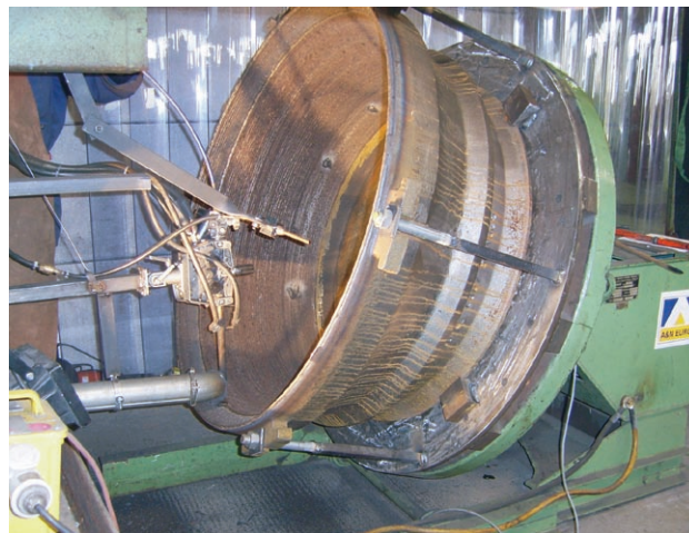
Figure 4. Regeneration of a crusher shell.
