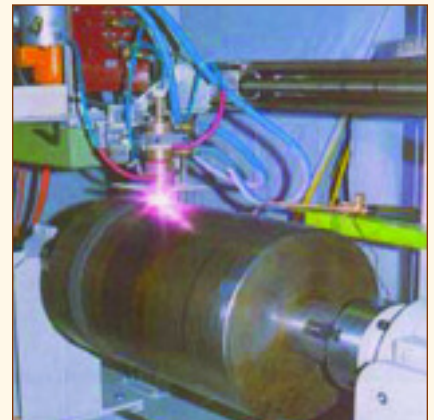
Fig. 1 — Plasma arc welding with powder containing an extremely high share of carbides.
